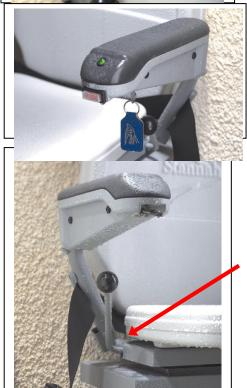
Check that the **red** on/off switch is switched off before you sit in the stairlift. You will find the **red** on/off switch located at the end of the armrest. The **red** on/off switch is on when the **green** light is lit.
