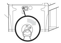
When the key and the on/off switch are in the on position, the light on the on/off switch will come on.
