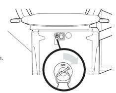
When the key and the on/off switch are in the on position, the light on the on/off switch will come on.
